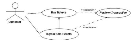
**Fig. 12** The use case diagram after five use case descriptions are read
